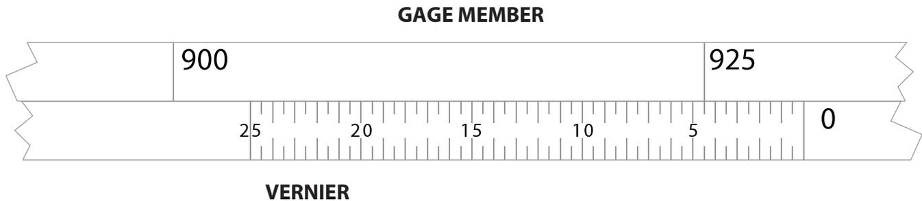
**Vernier Scale divides each graduation on Gage Member into 50 parts or .5mm**
